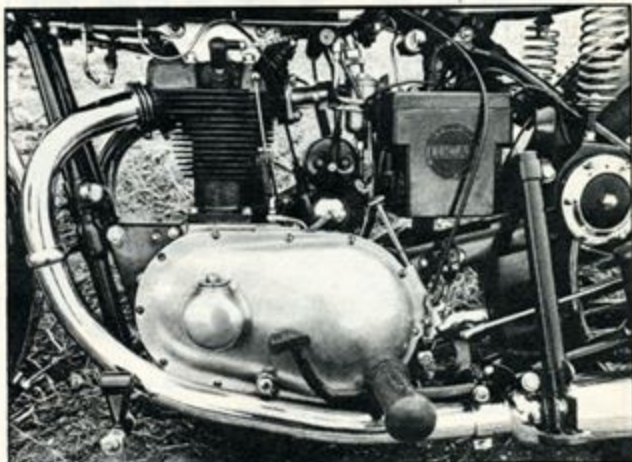
Drive side view of the 6/1 engine reveals partly exposed valve gear, oil feed to head, ingenious plunger and ratchet parking brake and patent spring-loaded side stand.
