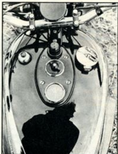
Tank top features include oil pressure indicator button (left), ammeter, lights switch and inspection lamp.
