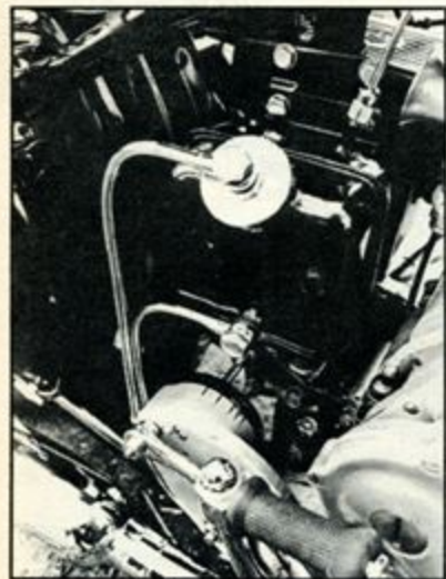
The pressurised oil filter housing is mounted just above the gearbox positive-stop mechanism.
